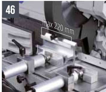
46 COBRA 352 NC 5.0 Special vice to reduce restpiece
