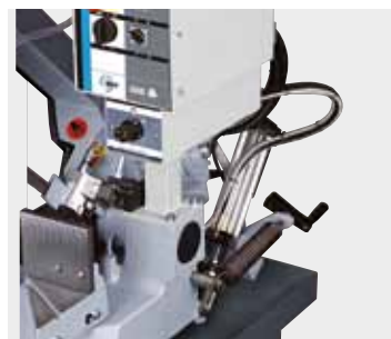
SHARK 281 - Cut Control System-Nachrüstsatz (kit to retrofit)
