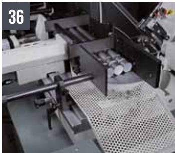
Device for bundle cutting w/guide to unload pieces cut (max 240x90 mm)
