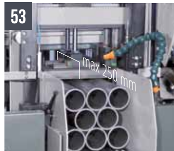
53 SHARK 230 NC HS 5.0 - Hydraulic vertical vices for bundle cutting (max 230x230 mm)
