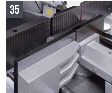
SHARK 332 NC 5.0 Special vice to reduce restpiece
