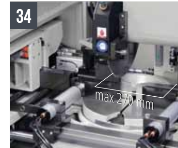
TIGER 372 CNC LR 4.0 / TIGER 402 CNC HR 4.0 Automatic head system with mechanical strokes adjustable in three position, 45° - 0° - 45°, equipped with special vices for reducing scraps.
