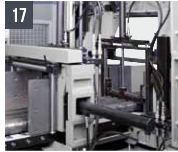
17 SHARK 310 CNC HS 4.0 - Hydraulic vertical vices for bundle cutting (max 310x310mm)
