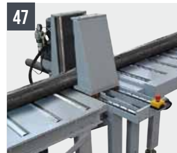
47 SHARK 640 CNC HS 4.0 Morsa allineamento barre
