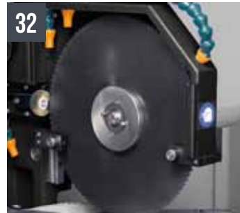
TIGER 372 CNC LR 4.0 (Ø max 105 mm) set of carbide guides
