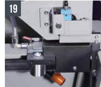
19 SHARK 310 CNC HS 4.0 Band deflection gauge
