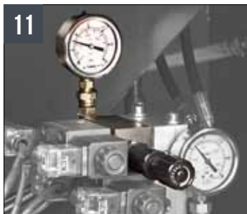
SHARK SXI evo Hydraulic vice pressure adjuster
