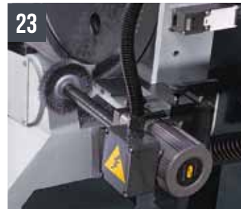
23 SHARK 422 SXI evo Motorized wire chip brush
