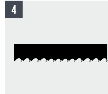
Band with electowelded hard metal plates
