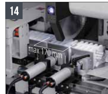
TIGER 402 CNC HR 4.0 - Set of comb jaws when equipped w/restpiece reduction min. (max70x70mm)
