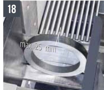
18 SHARK 310 CNC HS 4.0 Special vice to reduce restpiece
